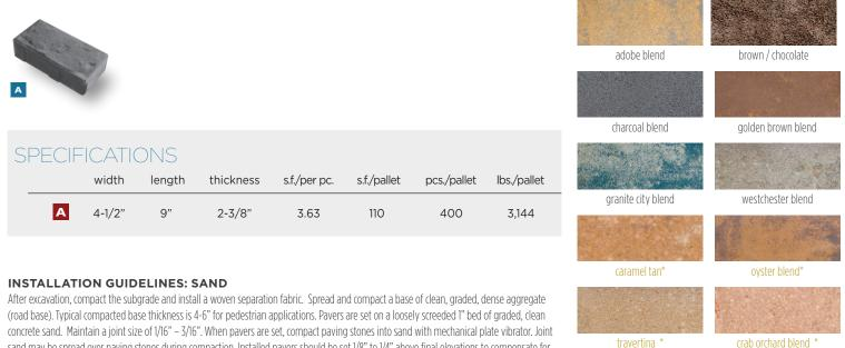
sand may be spread over paving stones during compaction. Installed pavers should be set 1/8" to 1/4" above final elevations to compensate for any potential settlement. Spread clean dry sand over surface and broom sweep to fill joints.
